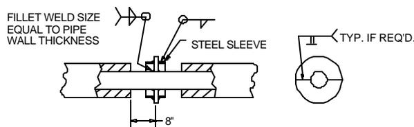
BELOW GROUND STEEL SERVICE PIPE ANCHOR
