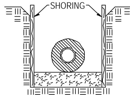
Organic soils or plastic clays and silts with high liquid limits may be encountered that are incapable of supporting the pipe. Remove the poor soil, and replace it with proper bedding soil to a depth that will provide a firm stable foundation.
