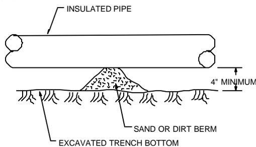
The material used for the berms should be in accordance with the recommendations provided in Section 7. If bags are used the bags should be cut open to allow proper compacting of the berm material. **Do Not** use wood or other degradable materials for berms.
