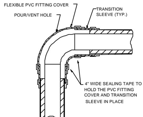
**NOTE:** It is important to tightly seal all seams with sealing tape. Gaps between the mold and insulation jacket will allow some of the rising pour foam insulation to escape. This could result in an incomplete pour and require mixing another small batch of insulation to complete the joint.
