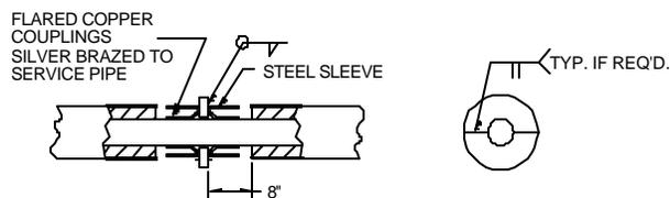
BELOW GROUND COPPER SERVICE PIPE ANCHOR
