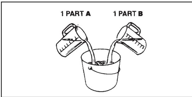
Immediately begin stirring the mixture. Stir vigorously for about 15 seconds. The insulation will begin rising in 15-30 seconds.
