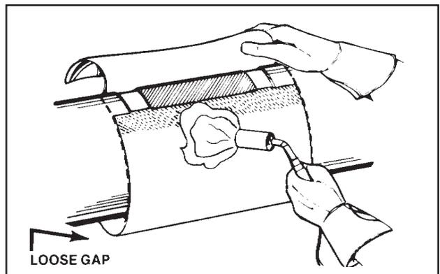
the sleeve before overlapping. Keep the torch in constant motion. **DO NOT burn the surface.**
