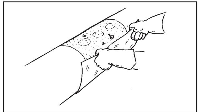
**NOTE:** The mold will be extremely hot. After removing the banding, peel the mold carefully off the insulation. If this is not done with care, the mold and the insulation will probably get damaged. If the mold sticks repeatedly, use additional mold
