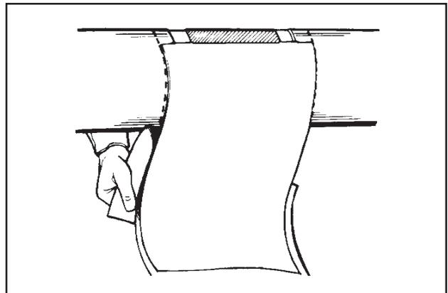
as the sleeve is wrapped around the joint.
