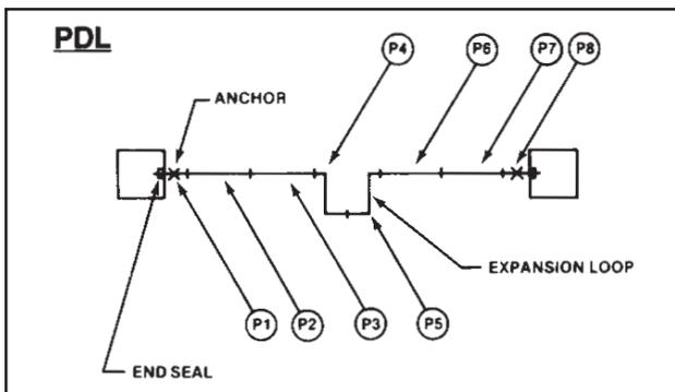
The part-drawing layout shows the location for each POLY-THERM assembly. Each assembly is marked with a number matching the number on the PDL drawing.
