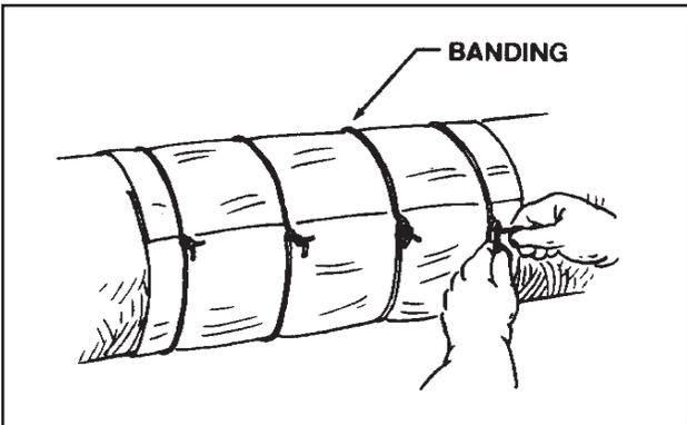
**NOTE:** It is important to fasten the mold tightly around the field joint. Gaps between the mold and the urethane polymer jacket will allow some of the rising insulation to escape. This could result in an incomplete pour and require mixing another small batch of insulation.
