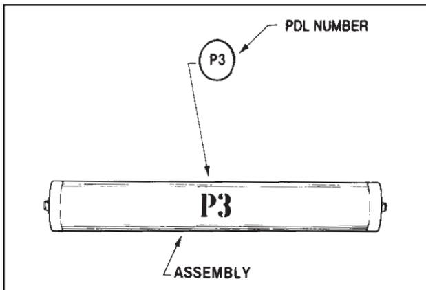
Laying assemblies in order next to the trench will simplify installation.
