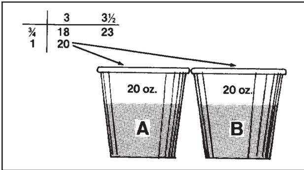
**DO NOT combine the two mixtures until you are ready to begin insulating the field joint.**
