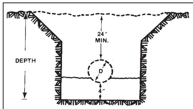
A minimum bedding of 4 inches must be raked uniformly along the entire length of the run. The bed of the run must be graded to a minimum slope of 1 inch per 40 feet. The bedding material should conform with the recommendations in the **Backfill** section of this manual (see Section 9.0).
