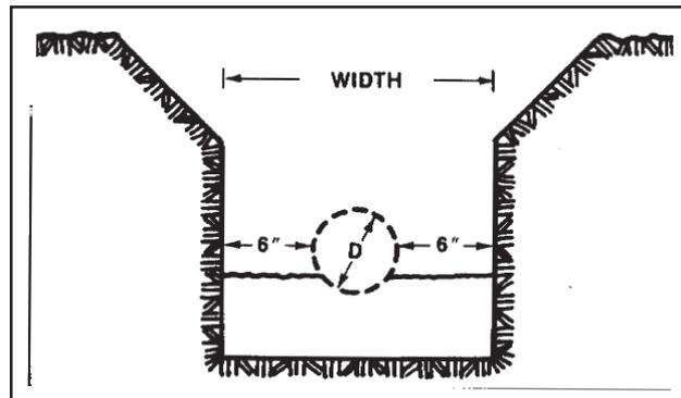
For multi-pipe installations, centerline dimensions can usually be found in the drawings.
