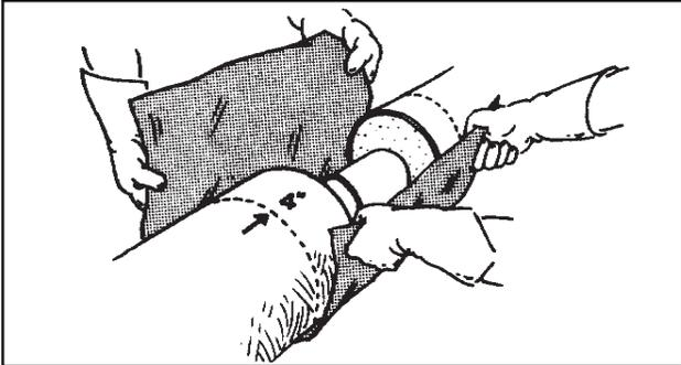
Tie a wire or rope band around the mold 2 inches from each edge. Use two more bands in the middle, evenly spacing all four.
