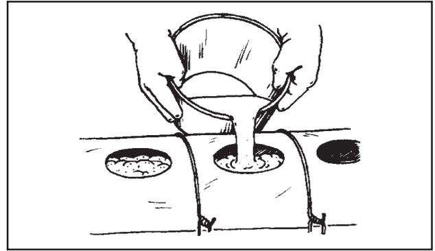
If the mold does not fill completely, remix small amounts of foam until it does. Also, adjust the amount of the mixture now needed for the remaining field closures.
