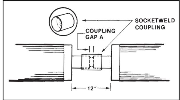
Refer to Table A for required coupling gap (gap A) between carrier pipes.
