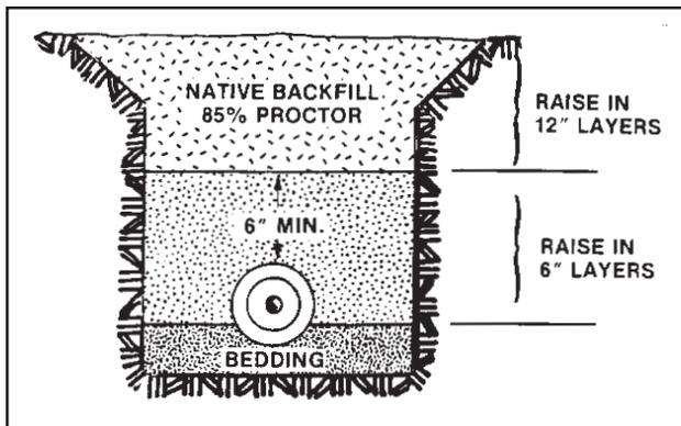
Under normal conditions, backfill to grade in 1-foot lifts and compact to 85% proctor. Native soil can be used, provided it is non-organic and all particles are less than 1 inch in size.
