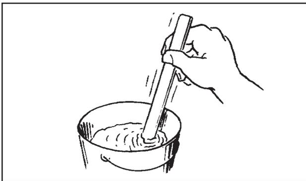
After 15 seconds of stirring, pour the mixture into the three holes at the top of the mold. The mixture will turn to foam and rise to the top filling the entire mold. The excess foam will push out through the top holes.
