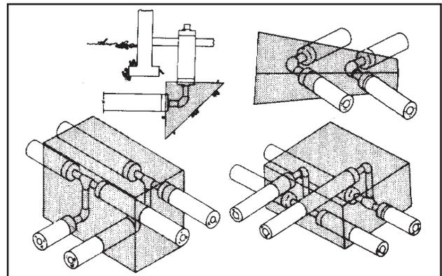
**NOTE:** For vertical risers, the trench bottom must be undercut and the entire elbow should be covered with concrete. The thrust blocks must bear against firm stable soil.
