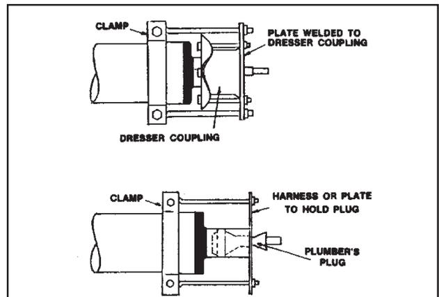
**NOTE: DO NOT** test the system at a pressure greater than 225 psi.
