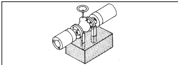
Typical examples of anchor blocks for normal fittings are shown.
