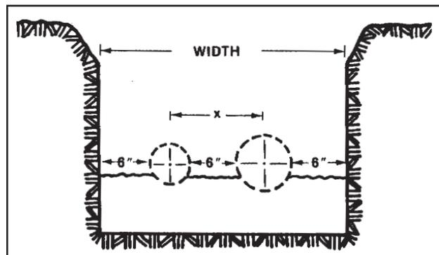
The total trench depth should allow for a 4-inch bedding, the conduit diameter and a minimum 24 inches cover depth above the conduit. See contract drawings for specific pipe burial depths. For depths less than 24 inches, contact PERMA-PIPE.
