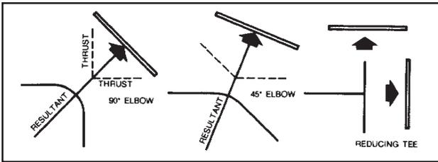
**NOTE:** Pour thrust blocks before hydrostatic testing of the pipe.
