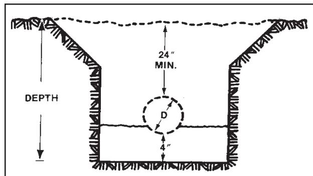
A minimum bedding of 4 inches must be raked uniformly along the entire length of the run. The bed of the run must be graded to a minimum slope of 1 inch per 40 feet. The bedding material should conform with the recommendations in the **Backfill** section of this manual (see Section 9.0).
