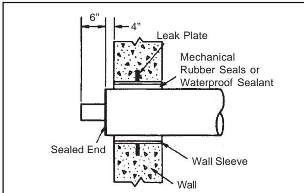
It is recommended that all building or manhole entries be sleeved and the annular space between the jacket and sleeve be sealed with either a mechanical rubber seal or a waterproof sealant. Wall sleeve and rubber seals are available from PERMA-PIPE.
