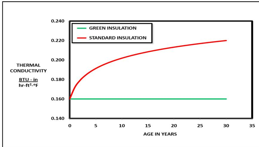
**Figure 2** - Comparison of aging and green foam insulations
